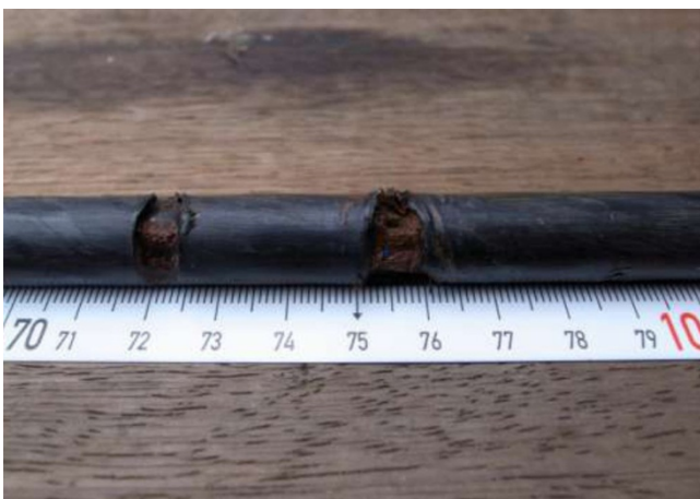
Figure 7-3-3. Photos of broken parts of the wire.
