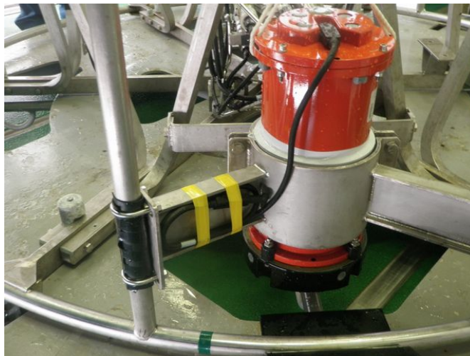
Fig 7.5-1 Mounting of LADCP on CTD System
