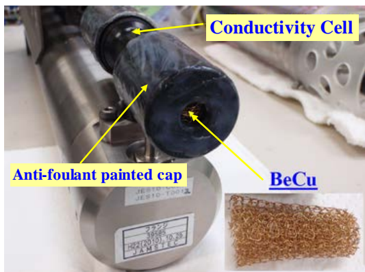
Photo 7.1.4-3 CT sensor attached BeCu on each end of the conductivity cell
