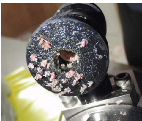
Photo 7.1.4-5 State of bio-fouling at the conductivity cell interior
