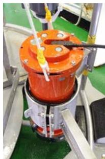
Fig. 5.14-1: Teledyne RDI Workhorse Sentinel 600kHz ADCP attached to the CTD frame
