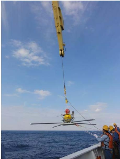
Figure 5.2.1 Photo of the operation of an OBEM deployment.
