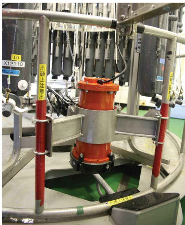
Fig 7.3.1 Mounting of LADCP on the CTD Frame
