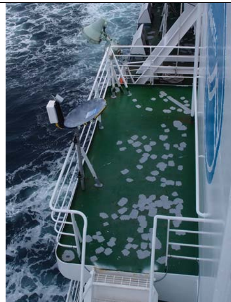
Fig. 6.1.3-2: The micro rain radar, installed on the starboard side of the anti-rolling tank.
