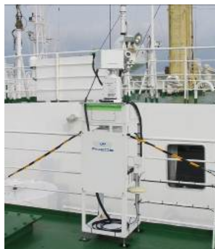
Photo 8.1.7-1 Solar tracker and telescope. The sunlight collected into optical fiber was introduced into the OSA that was installed in an observation room in the MIRAI.
