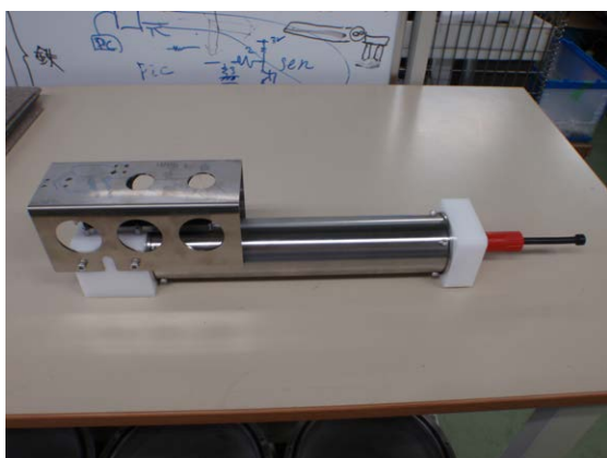
Fig6.1.3-1 JES10 profiler CTD sensor
