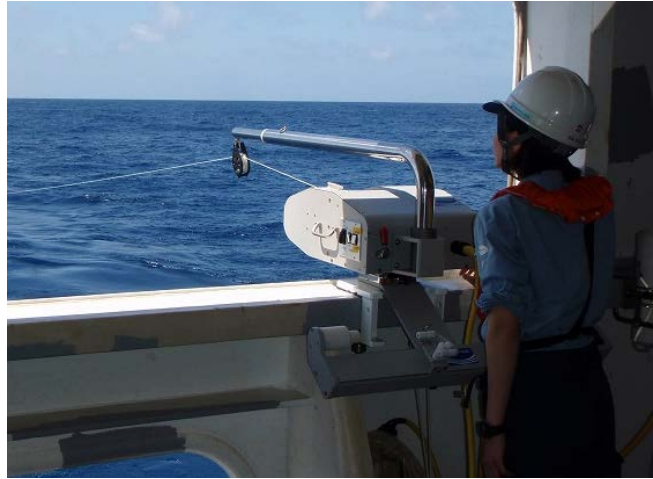
Figure 7.2.3-1: UCTD system installed and operated on R/V Mirai.
