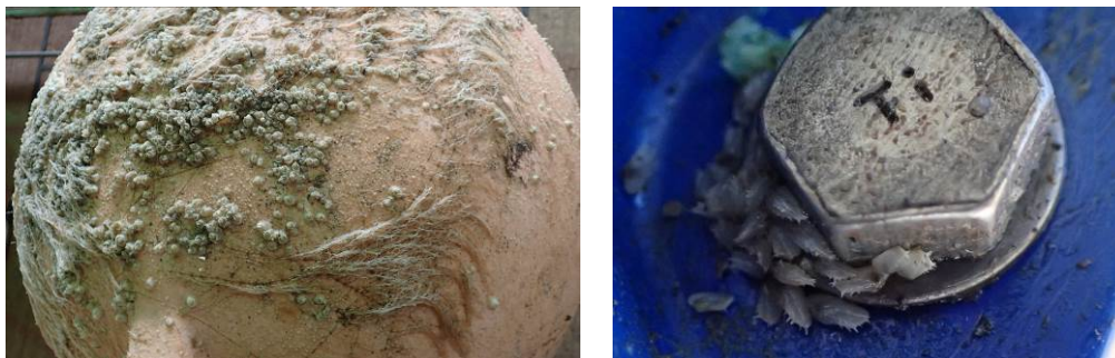
Fig. 4.20-2: The images of biofouling on the bottom-tethered physical oceanographic mooring at Station BCH deployed from September 2014 to September 2015. The left image shows biofouling on plastic float deployed at 96 m depth, and right image shows a small mass of tiny bivalves (?) attached around the bolt of ADCP deployed at 91 m depth.
