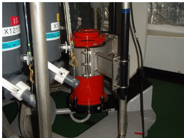
Figure 5.22-1: Mounting of LADCP on CTD System
