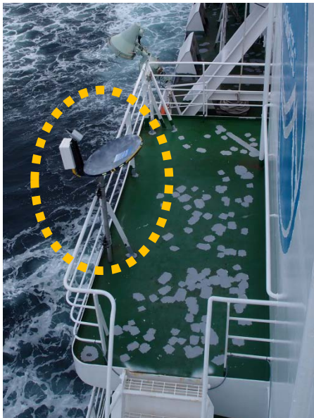
Fig. 5.5-1: Photo of the antenna unit of MRR
