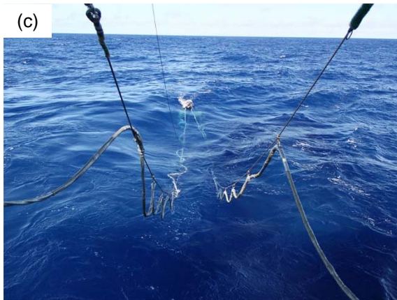
Photo 4.1.1. Photographs of source of MCS survey. (a) whole view of the air-gun array. (b) BOLT 2800LLX air-gun with 20 cu.in gun (looking from starboard side). (c) towing air-gun array.
