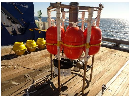
Figure 4.16-2-1. Picture of the sediment trap.
