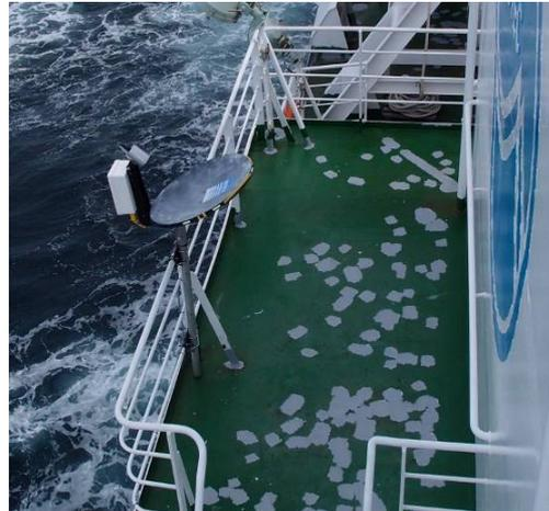
Fig. 6.8-2: The micro rain radar, installed on the starboard side of the anti-rolling tank.
