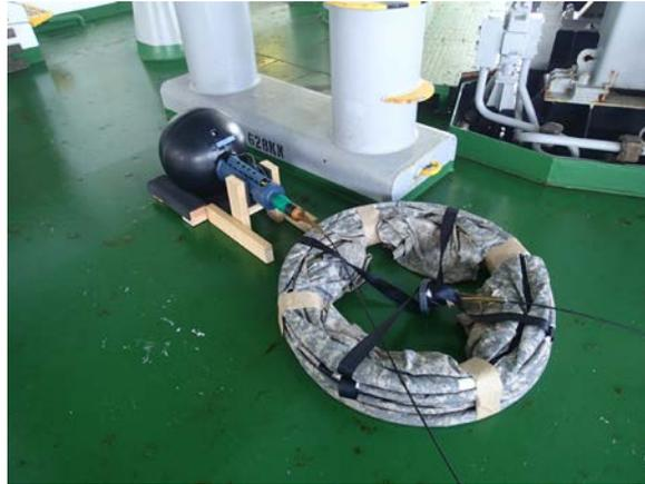
Fig. 6.2-1: External appearance of SVP-S drifter.
