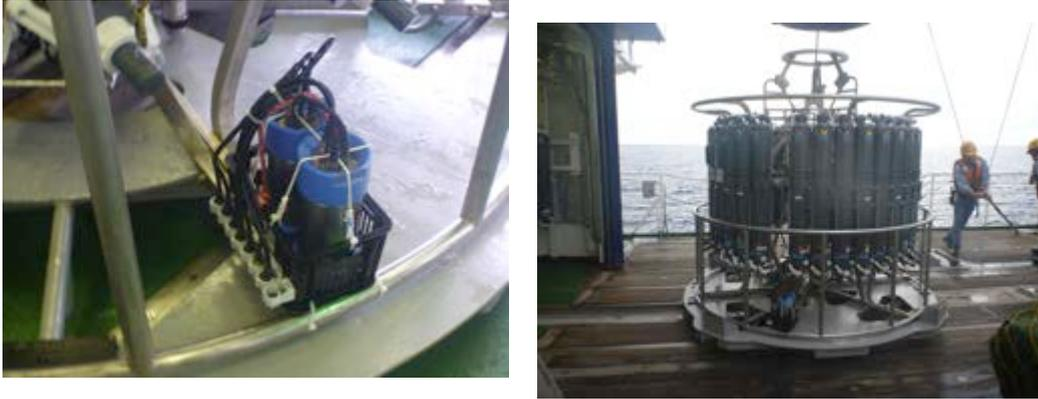
Fig. 6.12-1 In-situ pH/pCO<sub>2</sub>/ORP sensor
