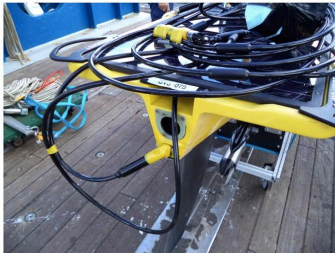
Fig. 6.4.-3 Thermistor chain and CTD sensor
