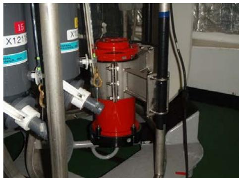
Figure 7.2.2-1: Mounting of LADCP on CTD System
