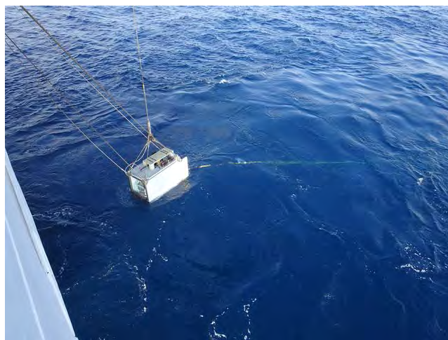
Fig. 5.2.3 Deployment of the EM deep-tow.
