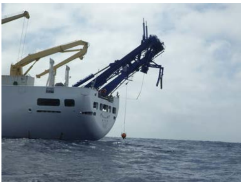
Figure 8d: Recovery of the BBOBS by the rope
