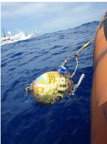
Figure 8c: Tying the floating BBOBS with a rope
