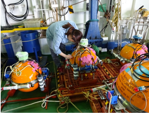
Figure 9. Ocean Bottom Pressure gauges (OBP)
