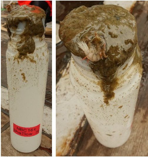
Figure 4.16-6. Sample bottle of upper sediment trap of NBC16t (#26) with clogged particles on the top of bottle. The clogging trouble probably occurs when the loophole of bottle water is closed by supply of aggregated particle mass from the bottom of trap cone.
