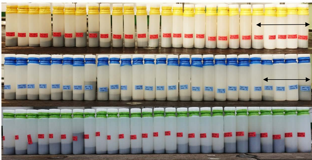
Figure 4.16-5: Recovered sediment trap bottles. Upper bottle line with yellow neck and middle line with blue neck is from the upper and lower sediment trap of NBC16t, respectively. Lower bottle line with pale green neck is from NHC16t. Left side is older (autumn 2016) and right end is this summer (Sep. 2, 2017). Arrows show the period for the clogging of trap cone.
