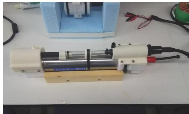
Fig5.24.2-2 JES10-Profiler with pump
