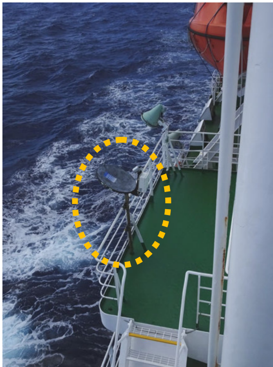
Fig. 3.10-1: Photo of the antenna unit of MRR
