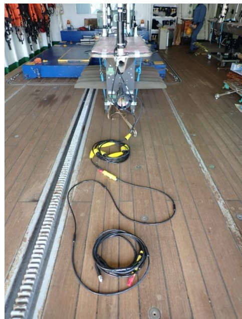
Fig. 5.3-3 Thermistor chain and tied CT/CTD sensors
