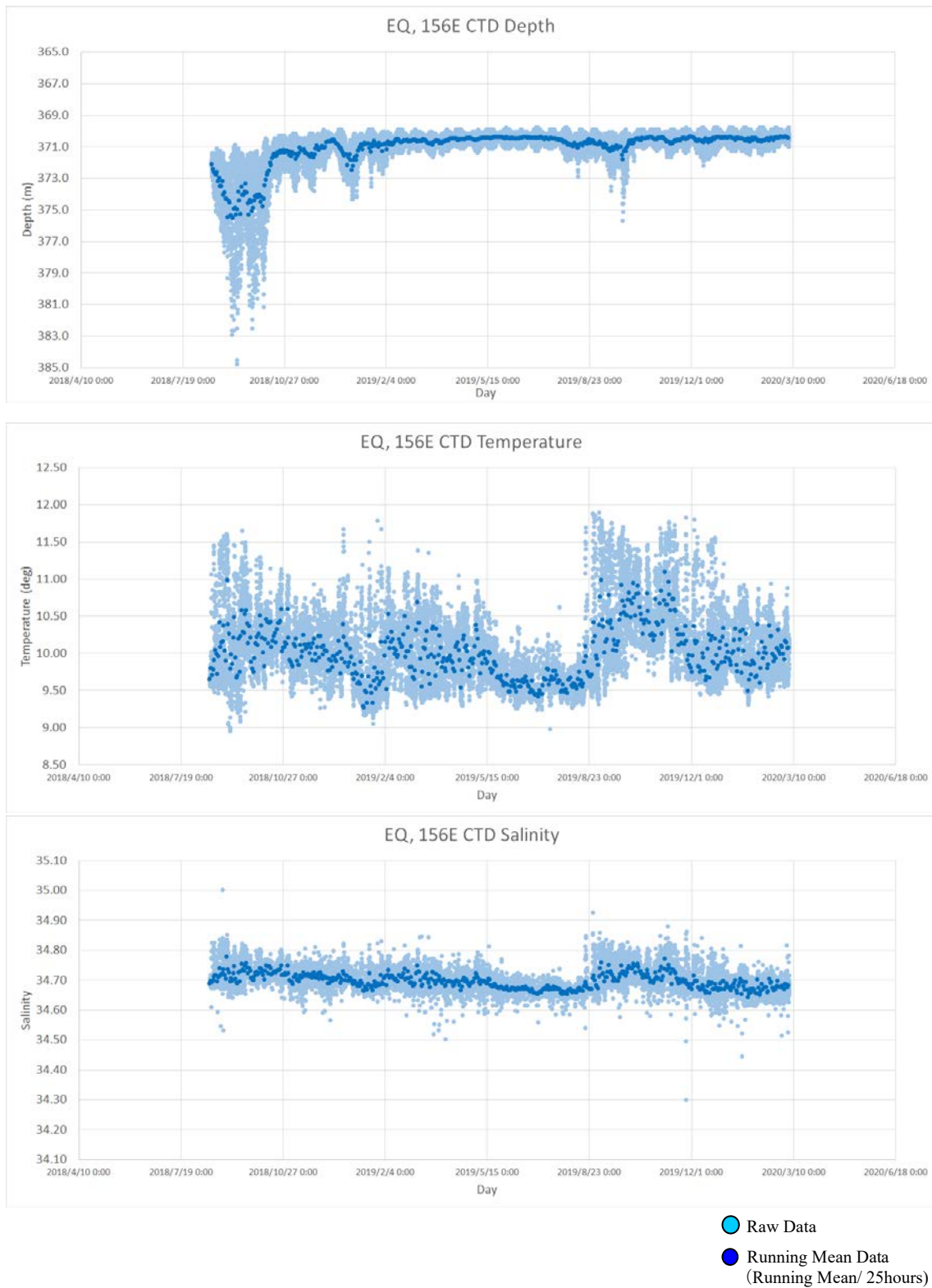
Fig. 5.2-3 Time-series of the observed pressure ( top panel ), temperature ( middle panel ) and salinity ( bottom panel ) obtained from CTD at Eq-156°E . (2018/08/17-2020/03/08)
