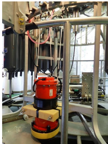
Figure 5.16-1: Mounting of LADCP on CTD System
