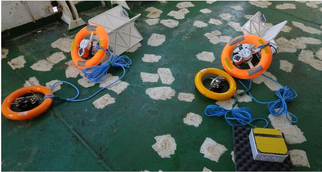
Fig. 5.6-1: The instruments used in the short deployment. Right ones are for Set 1, consisted of (upper) CARTHE, (center) Surpact, and (lower) IST micro chain. Left ones are for Set 2, consisted of (upper-right) CARTHE and (lower-left) Surpact. Note that the sensors of IST micro chain were not attached yet in this figure.
