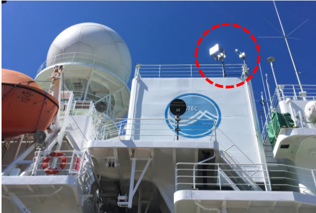
Fig. 5.5-1: Onboard LPM sensors. (Left) The location of the sensors, as designated by the red broken circle. (Right) The sensors. Right one (aft one) equipped wind protection element to reduce the effect of the wind, while left one (fore one) did not.
