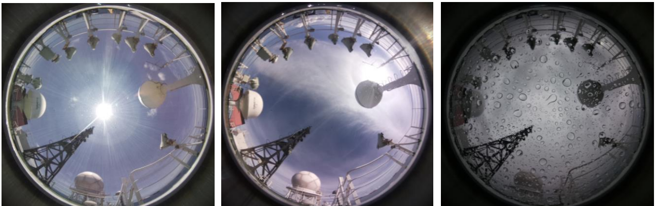
Fig. 5.11-3: Examples of the image from the whole-sky camera, at (left) a sunny moment, (center) a partly-cloudy moment, and (right) a raining moment.
