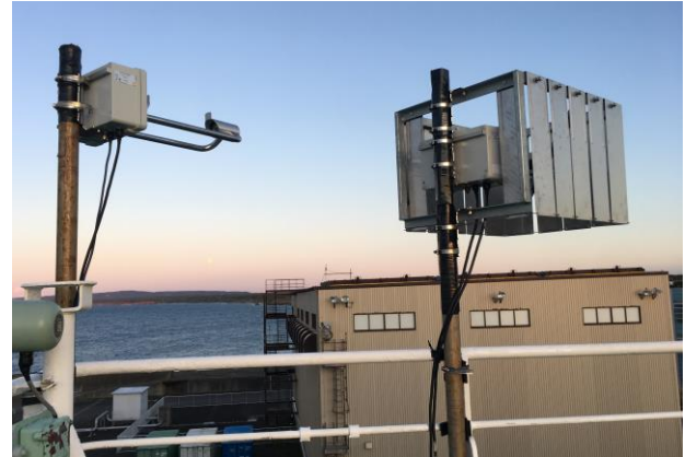
Fig. 5.5-1: Onboard LPM sensors. (Left) The location of the sensors, as designated by the red broken circle. (Right) The sensors. Right one (aft one) equipped wind protection element to reduce the effect of the wind, while left one (fore one) did not.
