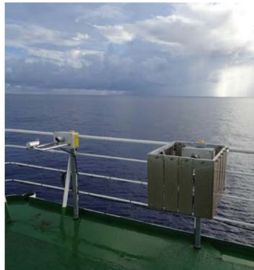
Fig. 6.14.1-1: Onboard LPM sensors. (Left) The location of the sensors, as designated by the red broken circle. (Right) The sensors. Right one (aft one) equipped wind protection element to reduce the effect of the wind, while left one (fore one) did not.
