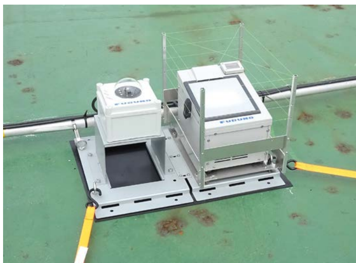
Fig. 6.15-1: Outlook of the microwave radiometer (right) and the whole-sky camera (left) installed at the roof of the aft wheelhouse.
