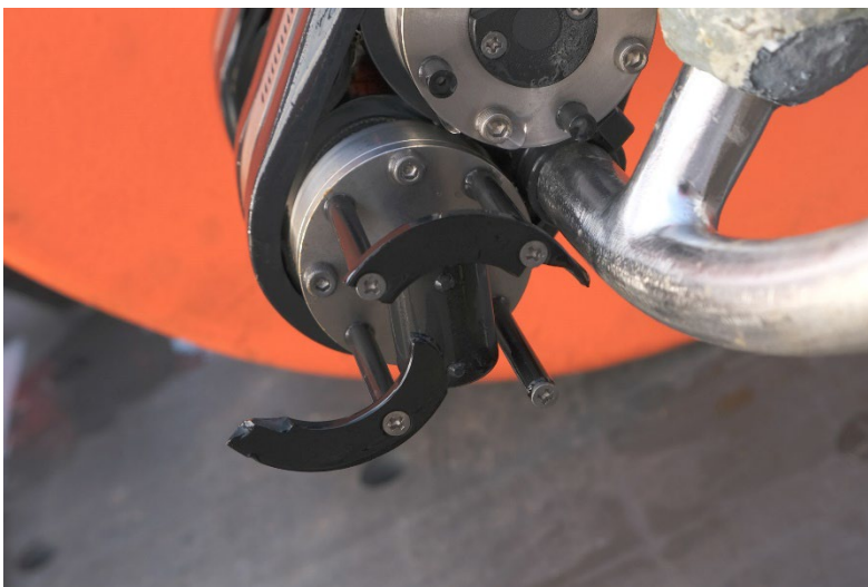
Figure 3.12.2-5: The photograph showing sensor guard of A7CT-USB (S/N613) recovered as the broken state, which had been attached on the mooring frame (lower part) of ice profiling sonar of NAP20t.
