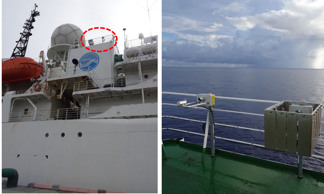
Fig. 2.2-1: Onboard LPM sensors. (Left) The location of the sensors, as designated by the red broken circle. (Right) The sensors. Right one (aft one) equipped wind protection element to reduce the effect of the wind, while left one (fore one) did not.
