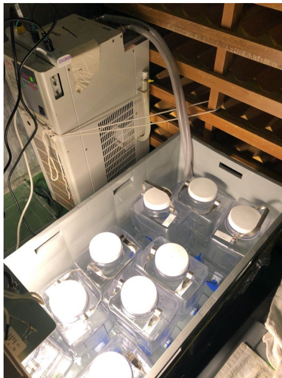
Photo 4.19.2: Temperature and light controlled incubation experiment system
