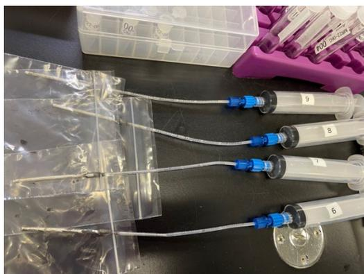
Figure 6.2-1: The Rhizon samplers, after they were used for the sampling during MR22-06C.
