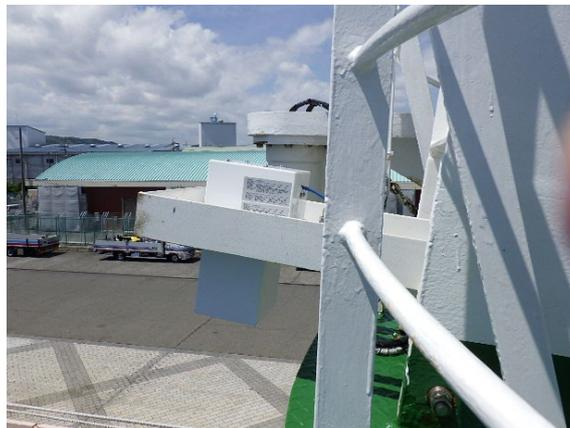
Figure 3.5-1: Microwave wave gauge installed at the bow.
