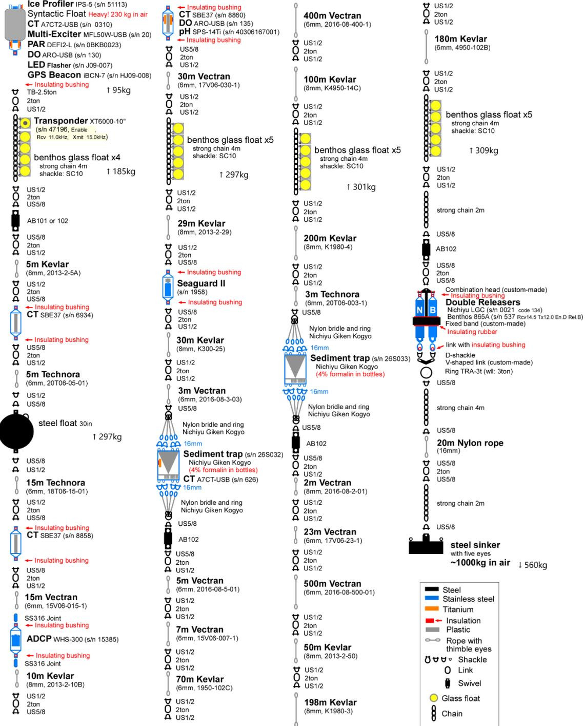
Figure 3.9.4-2: Diagram of the sediment trap mooring NBC21t for recovery.
