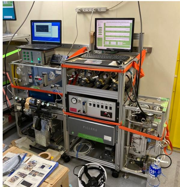
**Photo 2.6-1:** Flask sampling system (left) and continuous measurement system of the atmospheric CO<sub>2</sub>, CH<sub>4</sub>, and CO (right) based on a Cavity Ring-Down Spectrometer (CRDS) during MR22-06C cruise.
