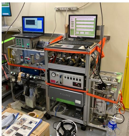
**Photo 3.11.3-1.** Flask sampling system (left) and atmospheric CO<sub>2</sub>, CH<sub>4</sub> and CO measurement system (right) based on a cavity ring-down spectrometer (Picarro G2401).
