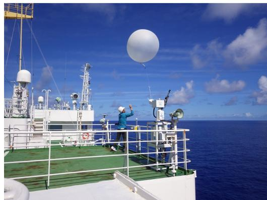
Figure 3.3.4-4 Launching of a balloon for radiosonde observation.
