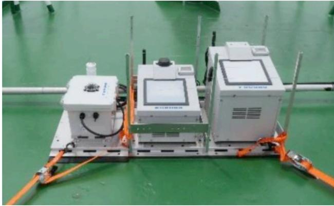
Figure 3.10-1 Outlook of the instruments installed at the roof of the aft wheelhouse; the microwave radiometer for the air temperature (right), microwave radiometer for the water vapor (middle), and the whole-sky camera (left).
