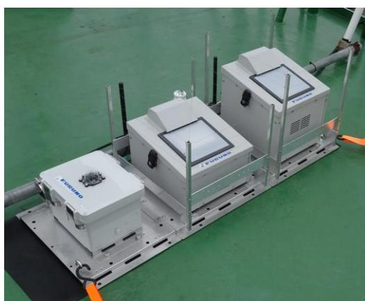
Fig. 5.10-1: Outlook of the instruments installed at the roof of the aft wheelhouse; the microwave radiometer for the air temperature (right), microwave radiometer for the water vapor (middle), and the whole-sky camera (left).
