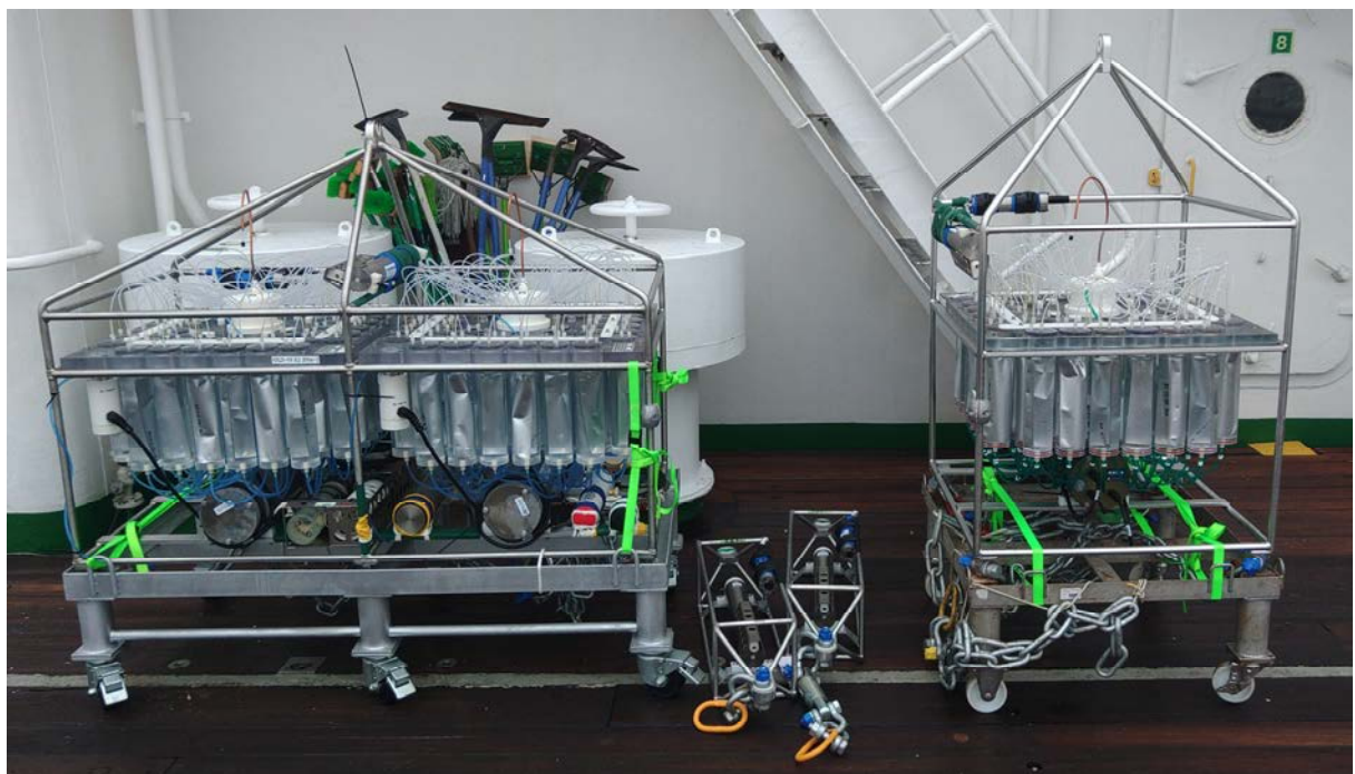
Figure 1 Remote Automatic Samplers deployed on 200m (left) and 300m (right).
