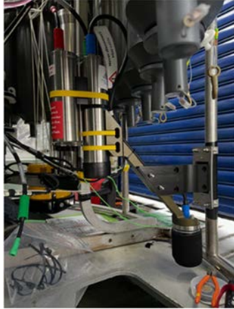
Figure 2.5.3-2. Photo of the UVP mounted on the CTD.
