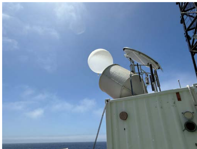
Fig. 2.1.5-1 Photograph of balloon released from the R/V Mirai shipboard launcher (taken by Dr. Maki Aita Noguchi)
