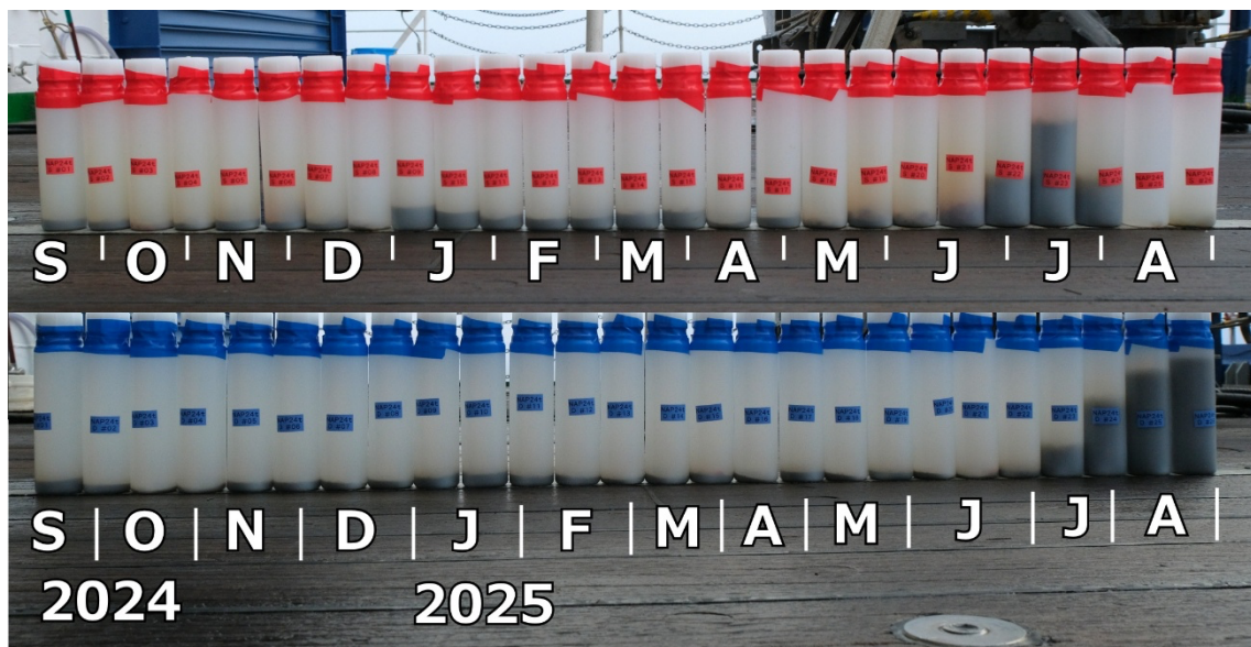
Figure 3.2.4.2 -6. The recovered sediment trap samples of NAP24t. The bottles with red and blue labels are from the shallow (nominally 200 m depth) and deep (1000 m depth) sediment traps, respectively.
