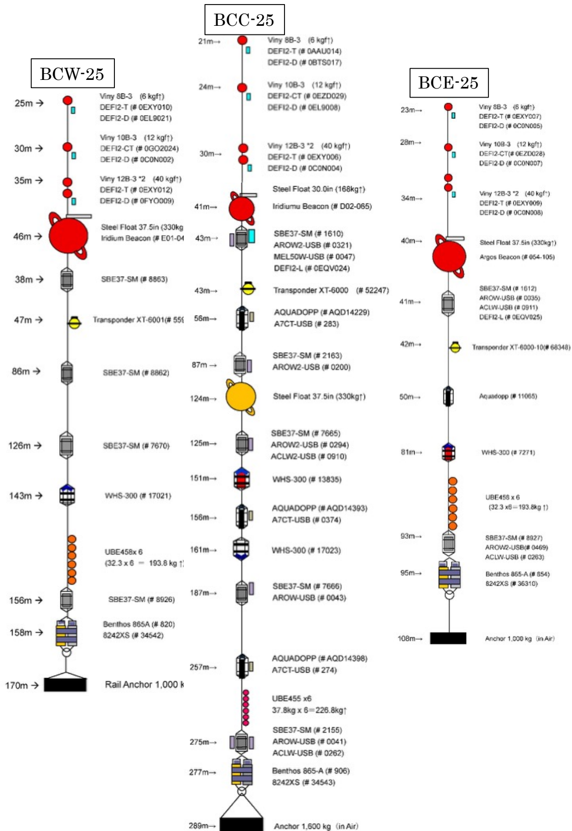
Figure 3.2.4.1-2: Deployed mooring diagrams.
