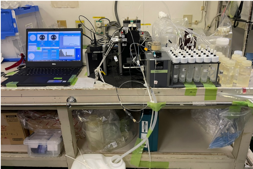
Figure 3.3.13-2. Shipboard analytical system for dissolved Aluminium determination using the programmable flow injection technique.
