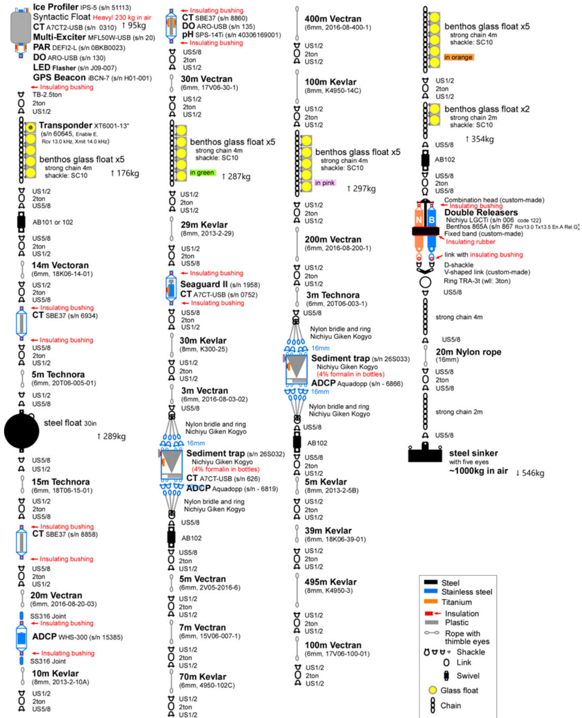
Figure 3.2.4.2 -3. The mooring design of NAP25t for deployment.
