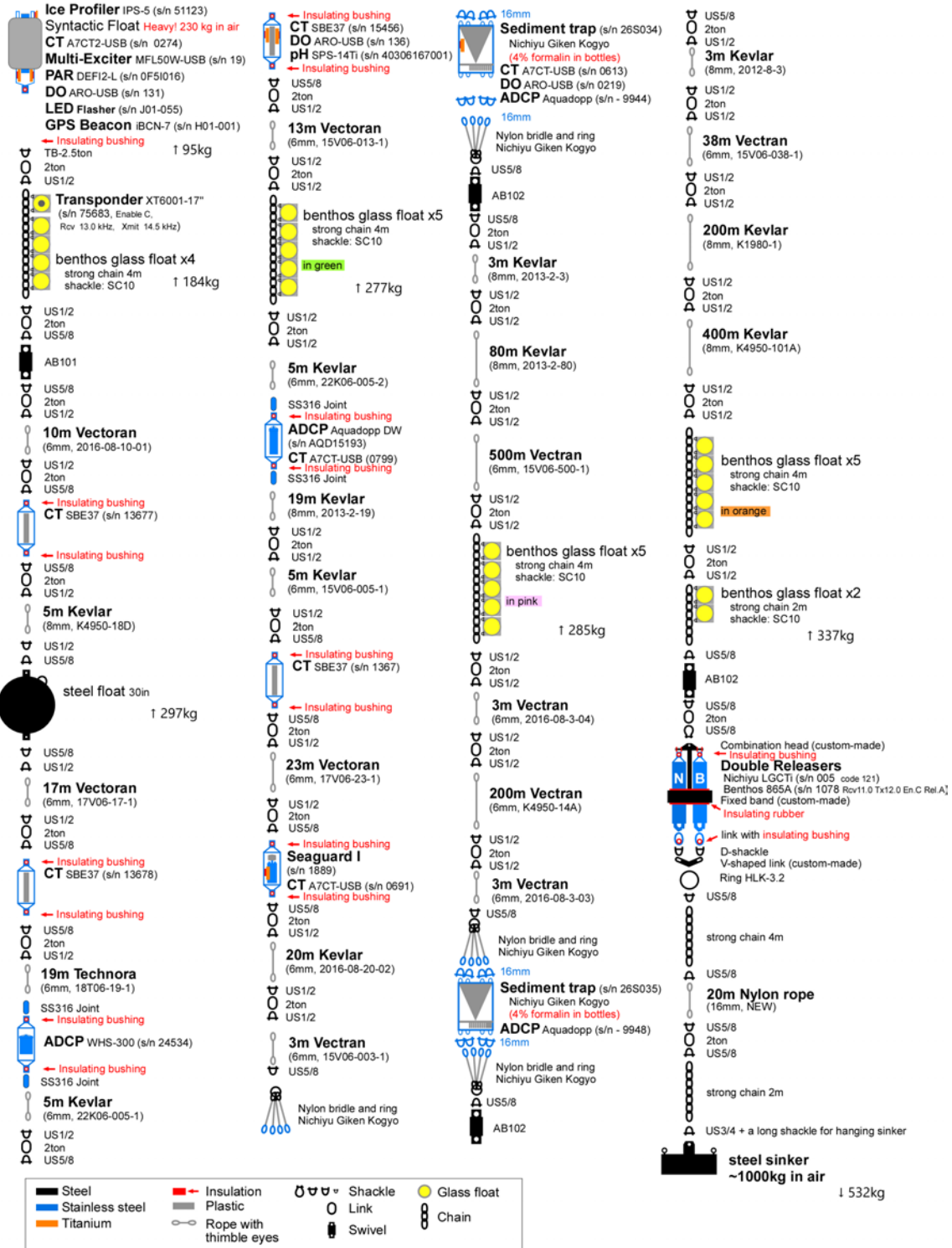
Figure 3.2.4.2 -2. The mooring design of NAP24t for recovery.
