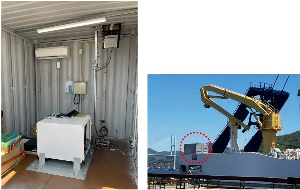
Fig. 6.13-1: Photographs of the ship-based water vapor and wind coherent lidar system. (Left) The lidar system inside the sea container. (Right) Sea container with the lidar system (circled in red) at the stern of the R/V Mirai.
