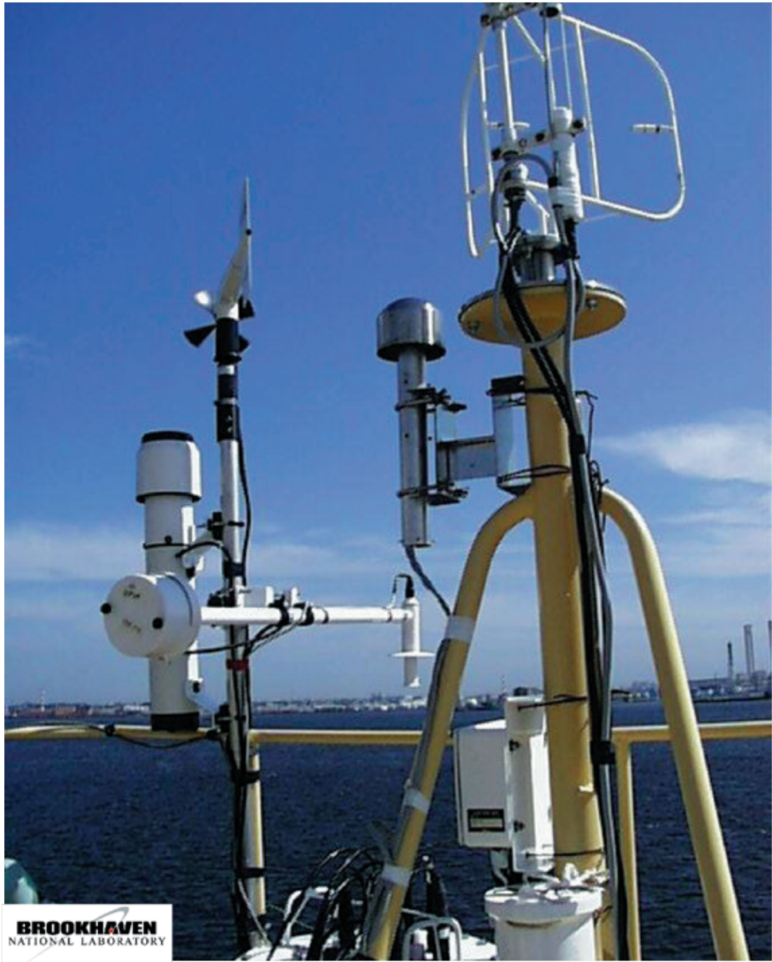
Figure 6.7-3. The Zeno meteorological observing system is shown to the left of the turbulence flux system. Shown are the wind monitor, rain gauge, aspirated T/RH and, just at the bottom of the figure, the Zeno data logger in its water proof canister. Out of view are the barometer pressure port, the optical rain gauge (ORG) and the sea snake at the bottom of the mast.
