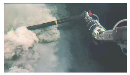
Figure 481B: Inserting the temperature and water sampling probe in the edge of the plume (image hdc20051010095910\_ 1)
