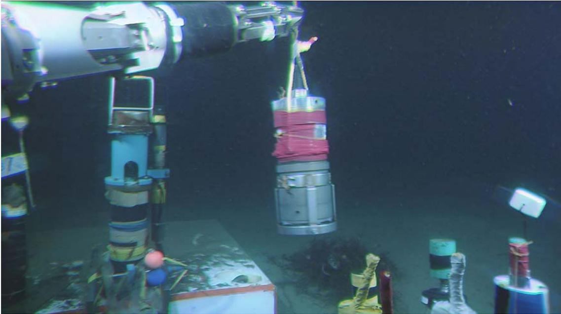
Figure 1. Pressure cylinder of the light source. Left square box is a basement of station OBB II.
