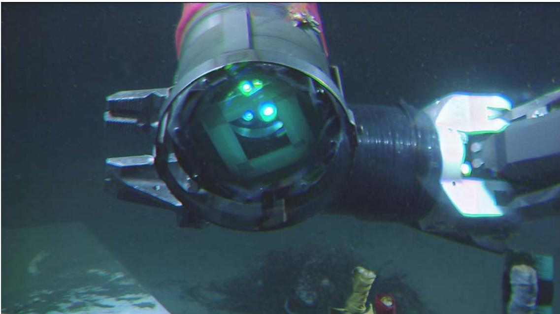
Figure 2. Sensing foil attached on the window (fixed by white tapes). Illumination of blue-green LEDs were confirmed before the deployment.
