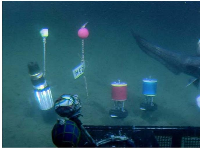
Figure 1. I-K type *in situ* feeding cores before setting (left) and after setting on the deep-sea floor (right).
