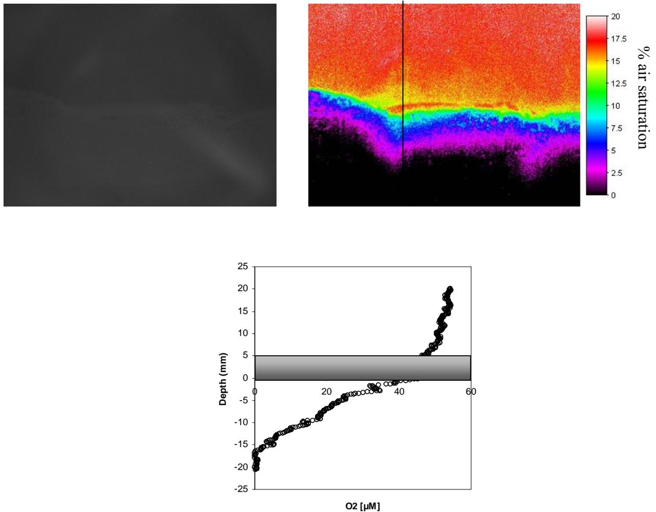
Fig 2 An example of a black-white image and the corresponding O<sub>2</sub> image. An example of an O<sub>2</sub> profiles extracted along the black line in panel 2 is included. The grey zone indicate the position of a fluff layer.
