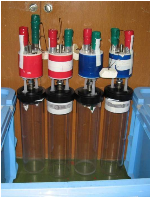
Figure 1. I-K type in situ feeding cores (G-2, G-y, C-2, and C-y cores from the left of the picture). Both G-y and C-y cores have 6 holes ( \phi = 1\text{cm} ) covered with plankton net on the top 1cm of the polycarbonate tube.
