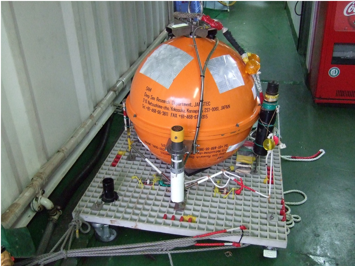
Figure 4 Recorder for the seafloor benchmark borehole seismometer.
