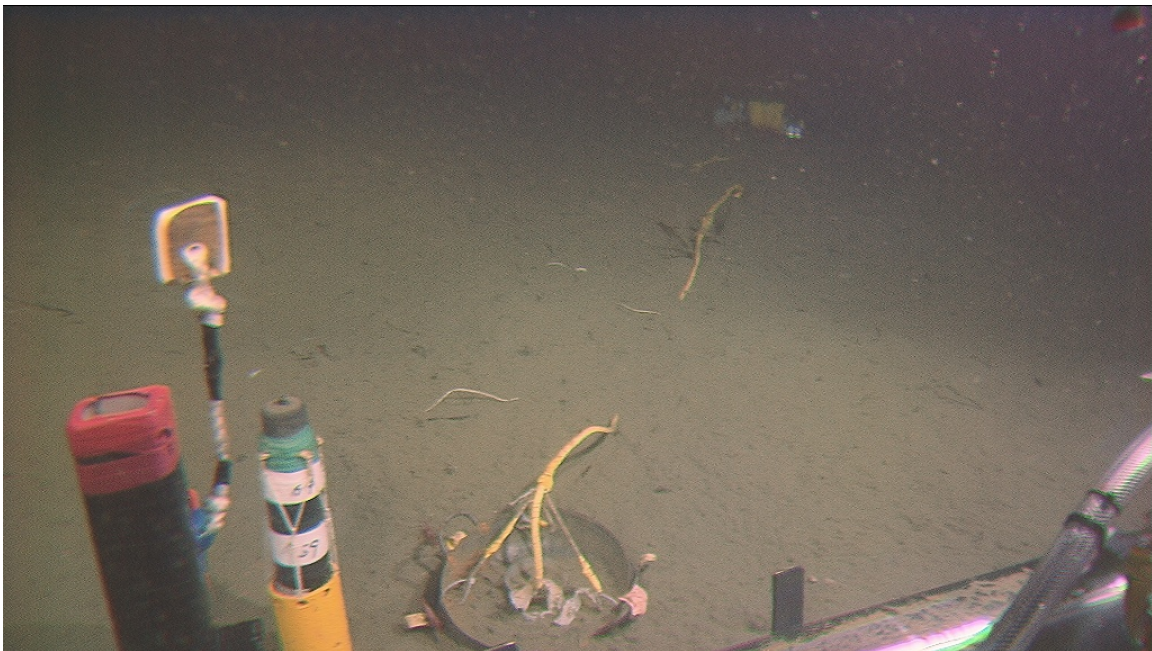
Figure 15. NABE-1 thermometer string in the seafloor benchmark hole before recovery (Dec. 12, 2006)
