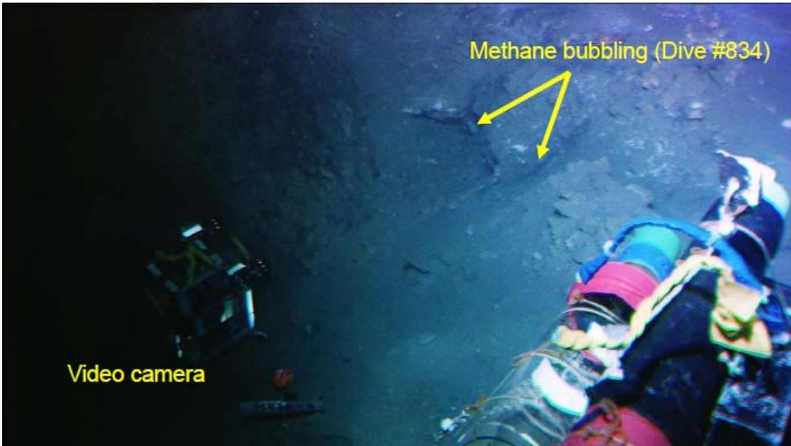
Fig. 23: A monitoring video camera system installed in front of the methane bubbling site discovered during Dive #834 (882 m).
