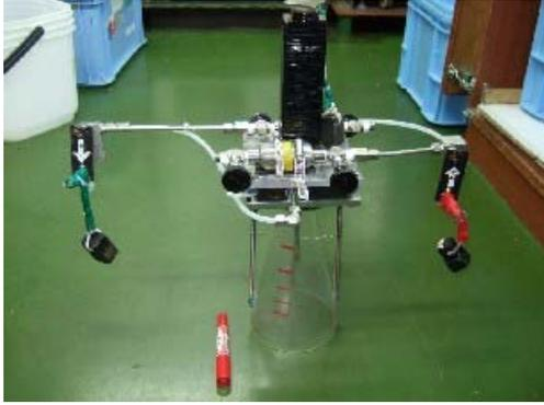
Fig. 5: M-type double vacuum sampler
