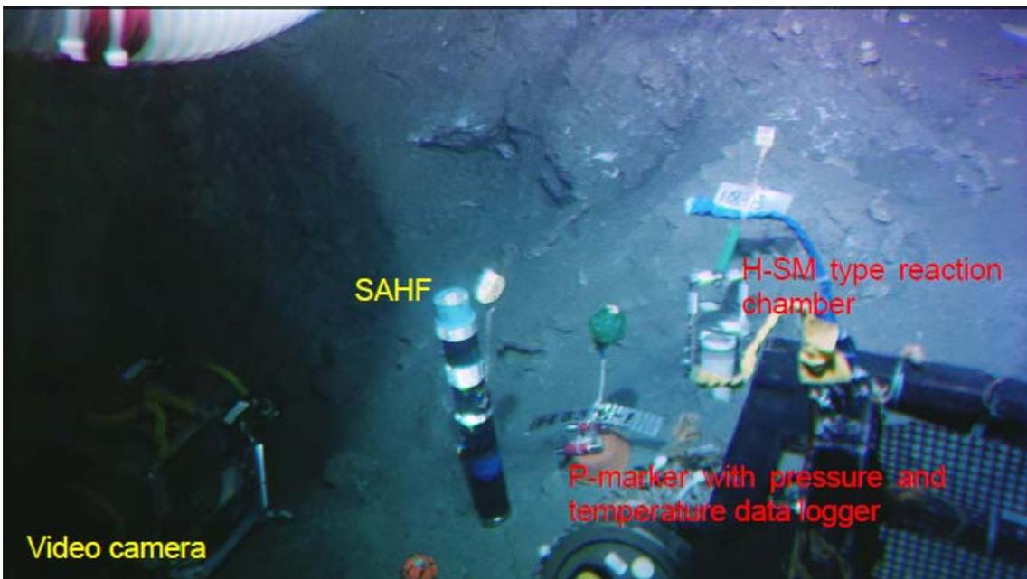
Fig. 24: Installed equipments adjacent to the methane bubbling site.
