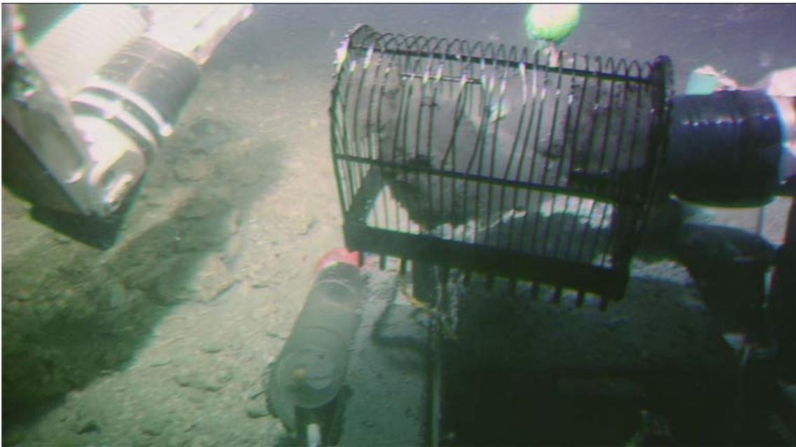
Fig. 25: Gas hydrate block in a wire net box for dissociation/dissolution test.
