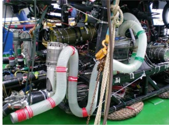
Fig. 6: Slurp gun
