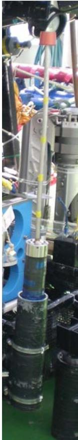
Fig. 2: Heat Flow Meter (SAHF)
