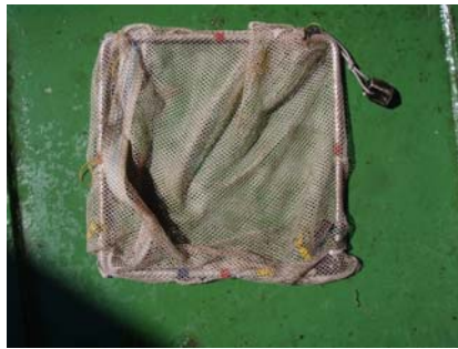
Fig. 9 Square wire (30cm x 30cm) with a net is useful in the collection of benthos. The net can be attached to the quadrate frame shown in Fig.9.
