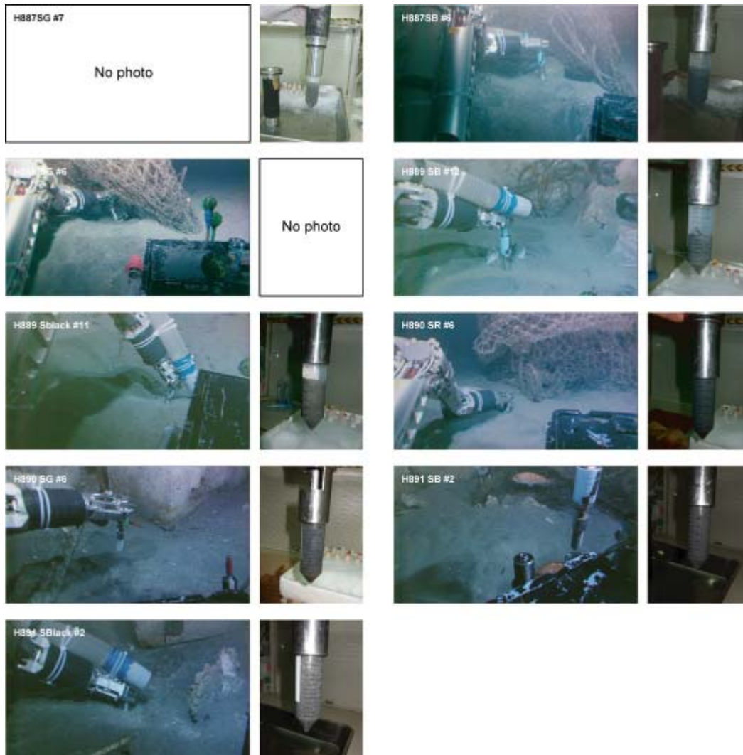
Fig. 24. Collection of sediment adjacent to whale fall by sterilized sediment sampler
