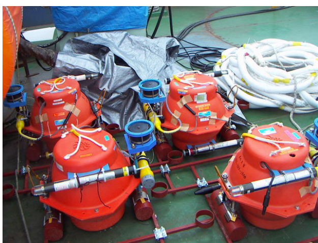
Fig. 3-2-3-1. Pre-deployed IESs with sinker.
