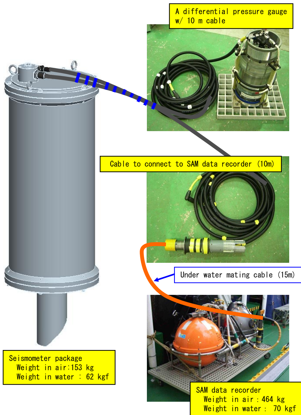
Figure 2 seismometer package and data recorder
