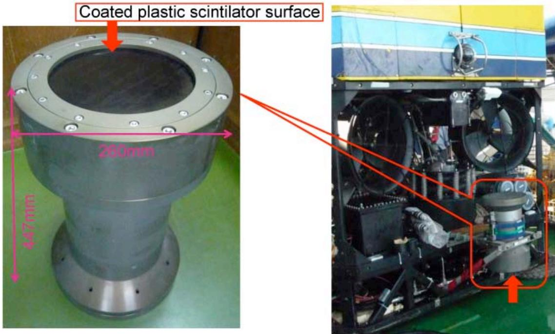
Plate 2-2: Rn-sensor (CRIEPI) and back view of HyperDolphin where the sensor was attached
