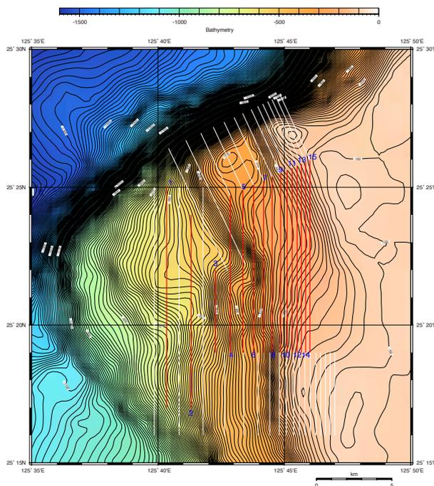
Figure 2: Bathymetric survey lines of the Miyako-Sone area (survey plan).
