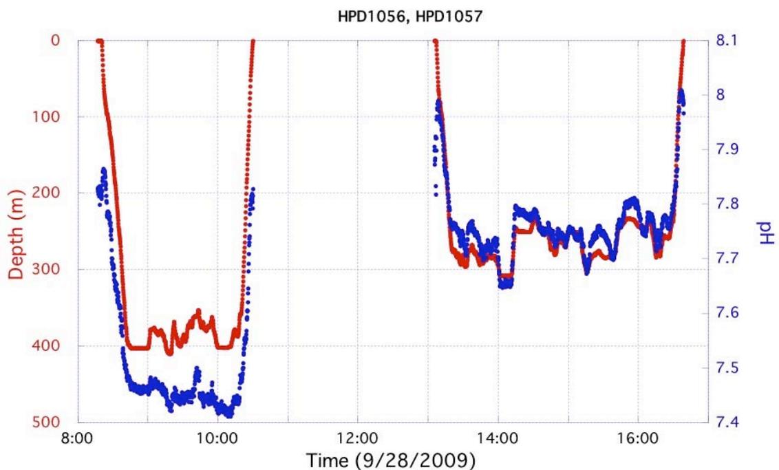
Figure 2-4: Raw data plot of pH sensor at the dives HPD#1056 and 1057.
