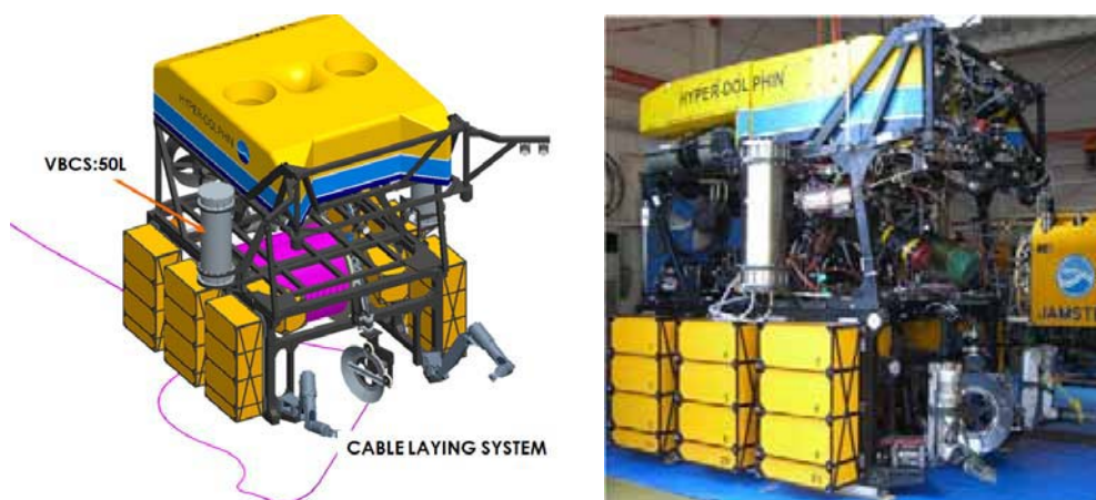
Figure 4 Cable Laying ROV
