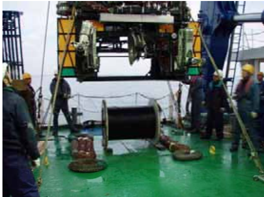
Photo 7 Recovery cable bobbin
