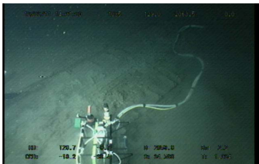
Photo 18 Pressure sensing system installation
