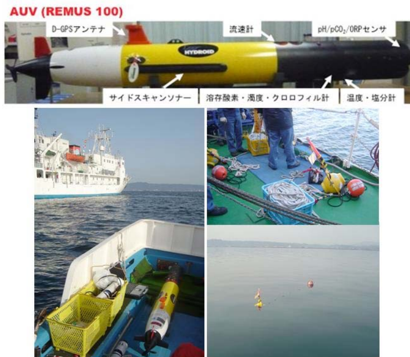
Fig.4 Deployment of AUV REMUS and Transponder mooring
