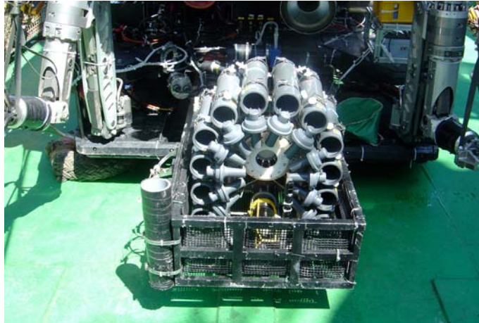
Fig.22 The Whole Assembly of CTD-Tytron System Mounted on the Vehicle
