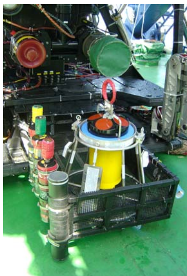
Fig.20 Photograph of ADCP before deployment, on ROV HYPER DOLPHIN
