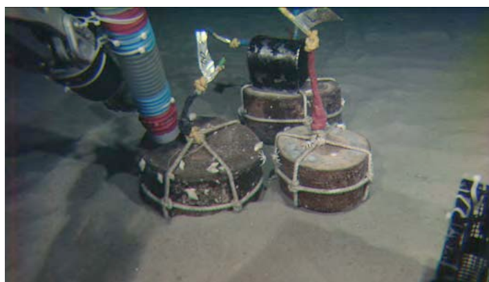
Fig. 4-1-5. Plankton sampling using suction sampler on the wood log (L-04).
