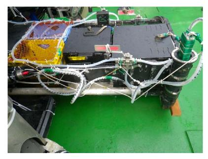
Arrangement of water sampler
