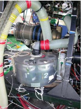
The rotary canister with canister bottles
