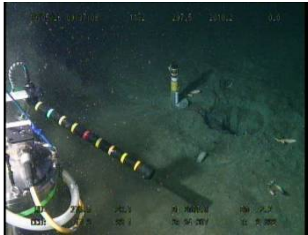
Photo 5 Penetrated burial casing at observation site A-2
