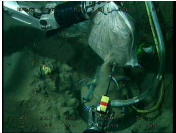
Photo 15 Post treatment of ground motion sensing system.
