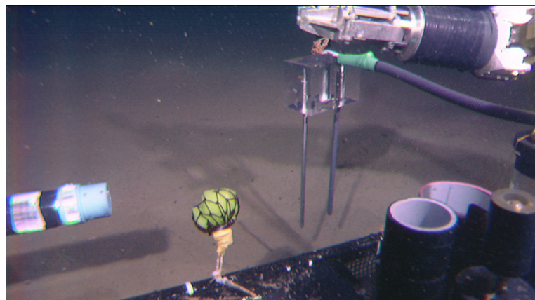
Fig. 10 TDR measurement on a muddy seafloor at St. 1141-3 (938 m).
