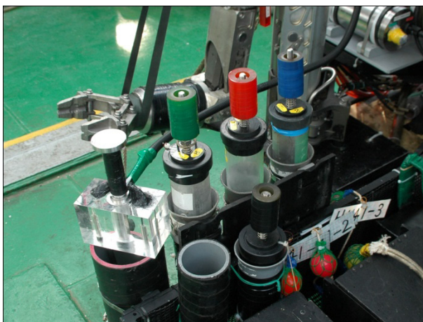
Photographs of MBARI type push corers and TDR sensor (having transparent acryl cubic).
