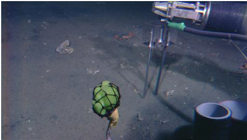
Fig. 6 TDR sensor into the seafloor by manipulator
