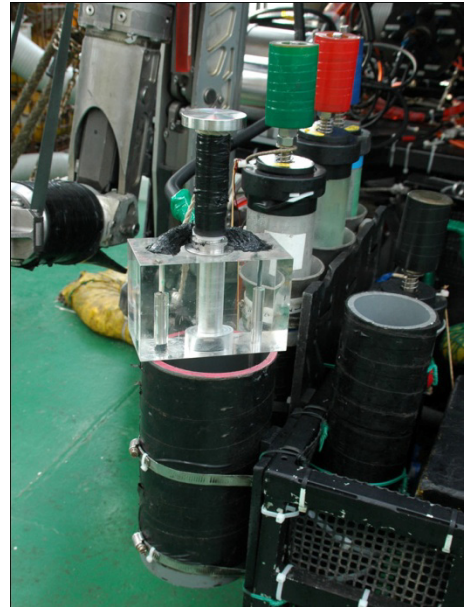
Above: Data logger for TDR sensor. It is located behind the sample basket. Right: Close up photograph of TDR sensor.
