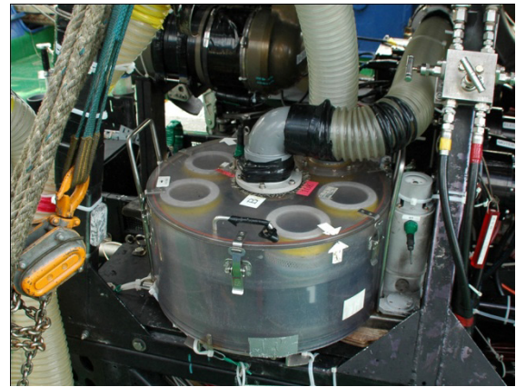
Left: Slurp Gun with 6 canister bottles system. Right: Close up photograph of 6 canister bottle system. This, each canister bottles were sealed by mesh cover.
