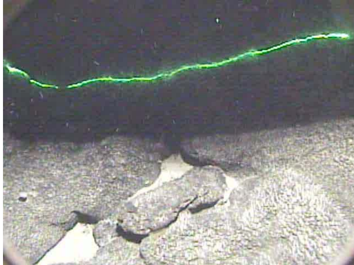
Fig. 13 Image captured during HPD#1145. The upper portion of the image is used to generate bathymetry while the lower part of the image is illuminated and contains colour information
