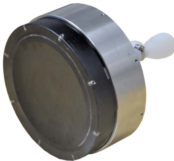
Fig. 5 Acoustic probe developed to measure manganese crust thickness
