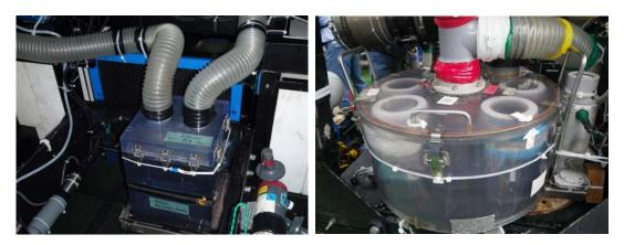
Cubic canister (left) and rotary canister (right)
