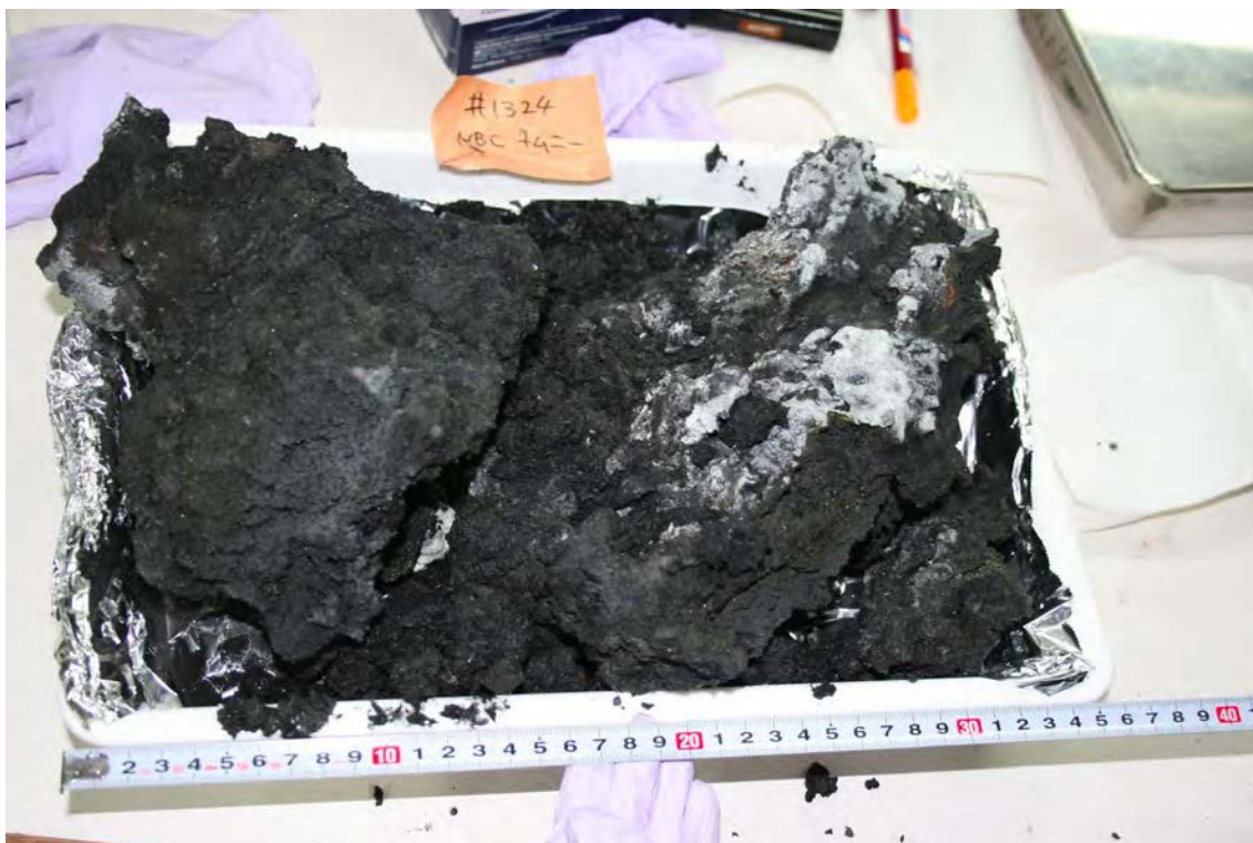
Fig. 1. Sample #1324R01 taken from a chimney in the cruise #1324. The sample is composed of fine muddy sulfides with outer white part probably of quartz.
