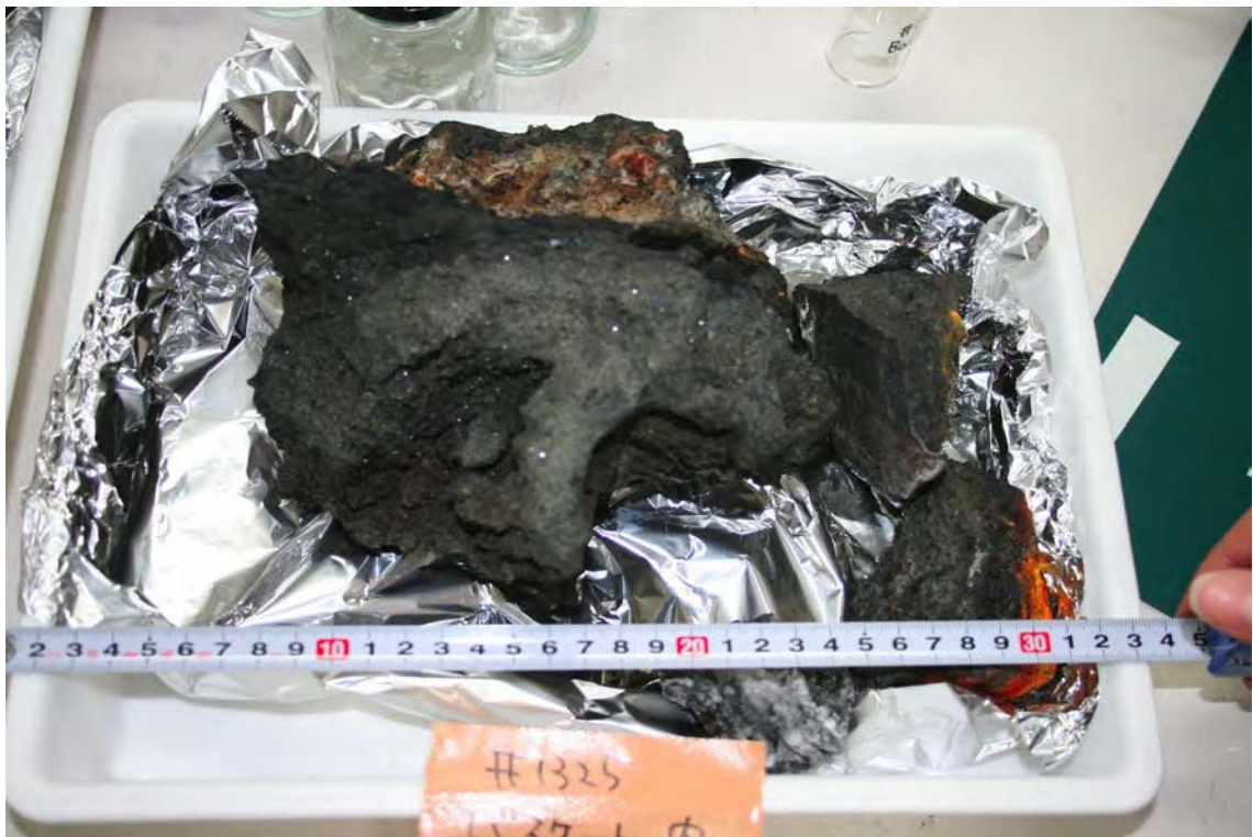
Fig. 2. Samples #1325R01-1 (upper, left), 1325R01-2 (upper right) and 1325R02 (lower) taken from a base of chimney in the cruise #1325. The sample is composed of
