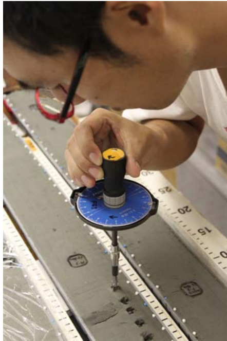
Figure 3.4-10. Vane shear test (Photograph was taken during the KH-10-3 cruise of R/V Hakuho-maru. The tester is Mr. Otsuka from AORI, University of Tokyo.)
