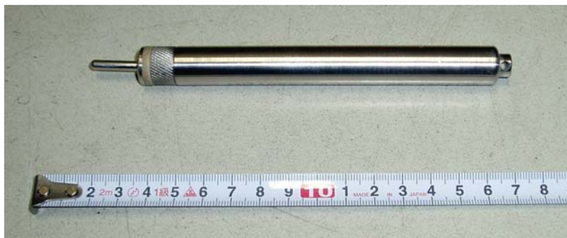
Figure 3.4-2. ANTARES Miniaturized Temperature Data Logger (MTL).
