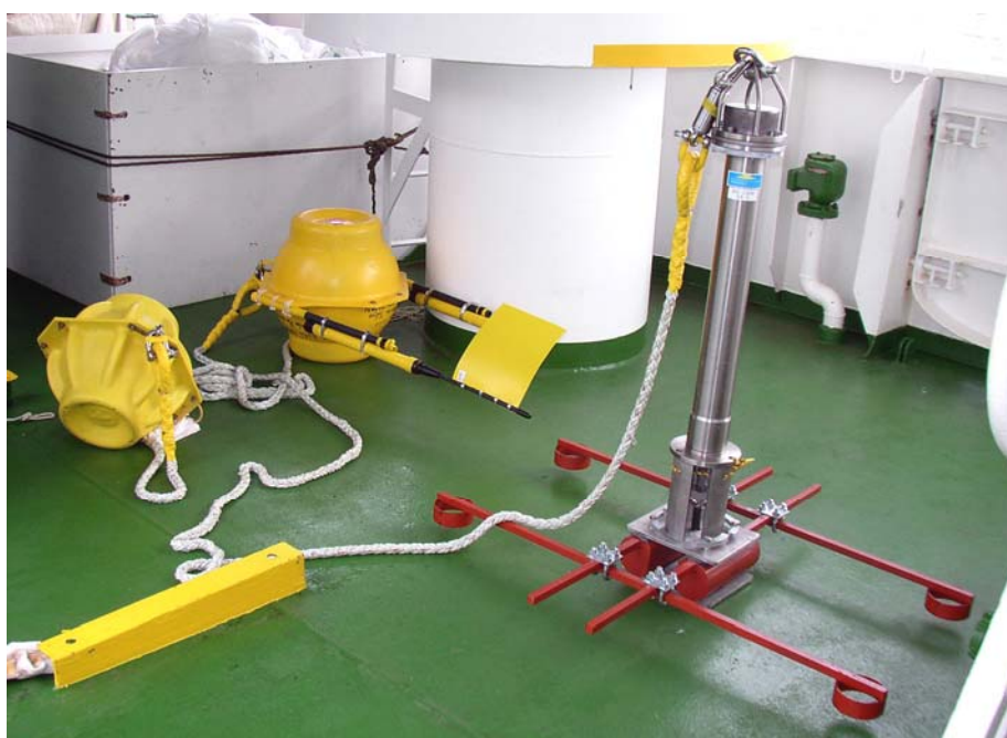
Figure. 3.4-6. Pop-up water temperature measurement system (PWT).
