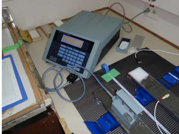
Figure 3.4-8. Thermal conductivity measurement on the sample NT11-23 PC01 with QTM-500.
