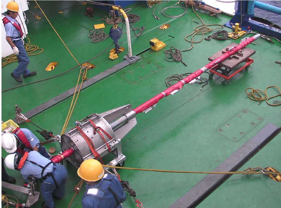
Figure 3.4-4. HFPC with compact temperature data loggers (MTLs).
