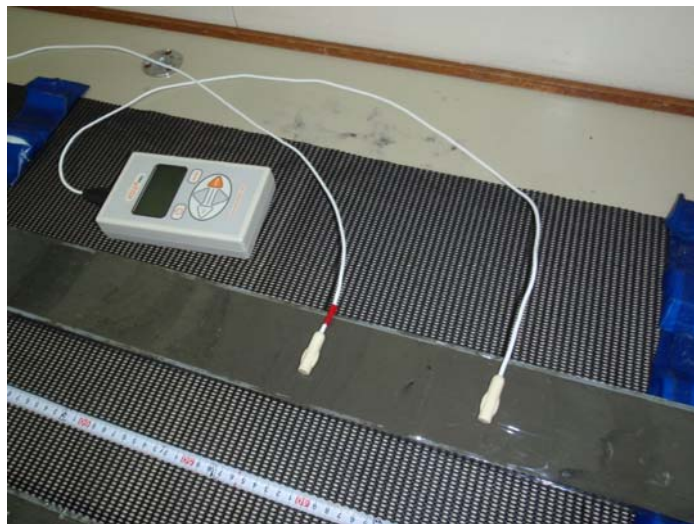
Figure 3.4-9. Thermal conductivity, heat capacity and thermal diffusivity measurements on the sample NT11-23 PC01 with dual probes of KD2 Pro.
