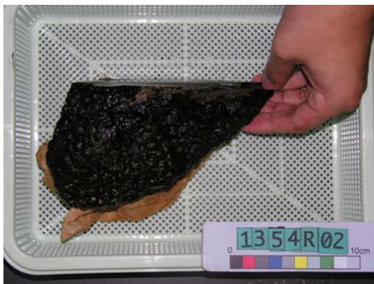
Fig.21. Surface-view photo of manganese crust sample, HPD#1354 R2
