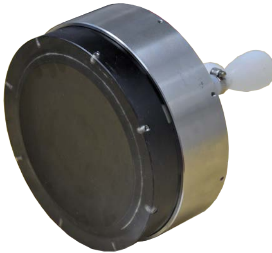
Fig. 6 Acoustic probe developed to measure manganese crust thickness
