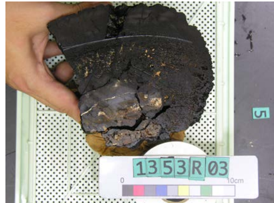
Fig.20. Side-view photo of manganese crust sample, HPD#1353 R3
