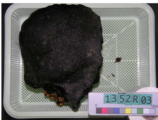
Fig.17. Surface-view photo of manganese crust sample, HPD#1352-R3
