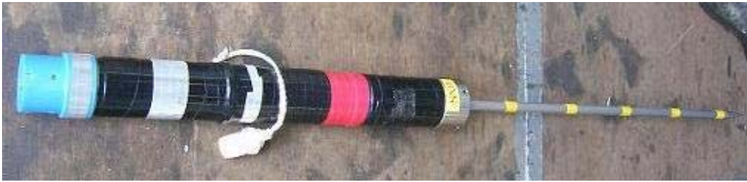
Figure 2. Stand-Alone Heat Flow meter (SAHF)
