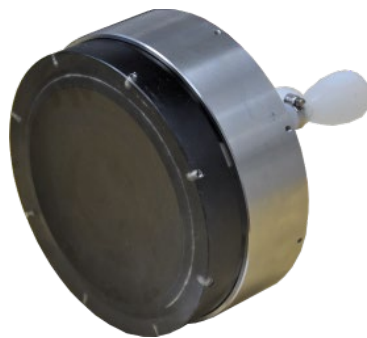
Fig. 3 Acoustic probe developed to measure manganese crust thickness.
