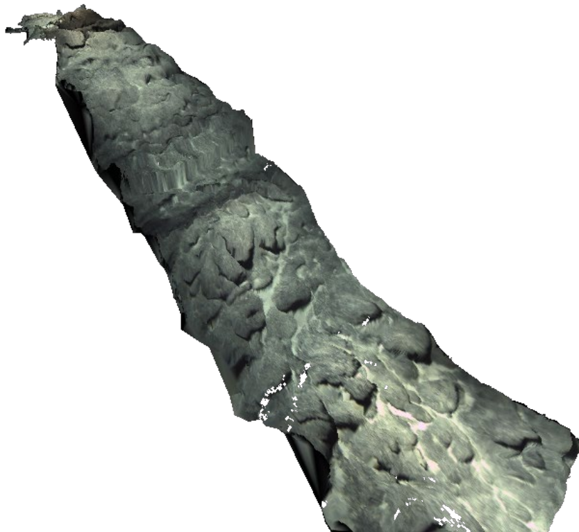
Fig: 23 3D reconstruction in colour using HPD#1540 data at depth 1704m
