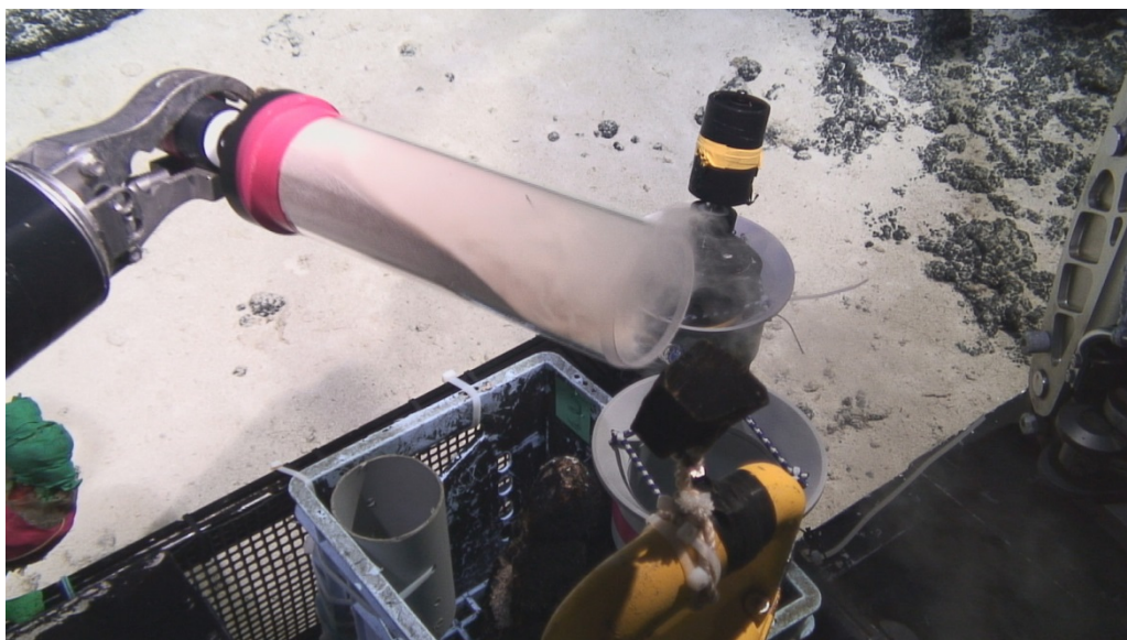
Fig: 27 Photo of push corer sampling of HPD#1540C01
