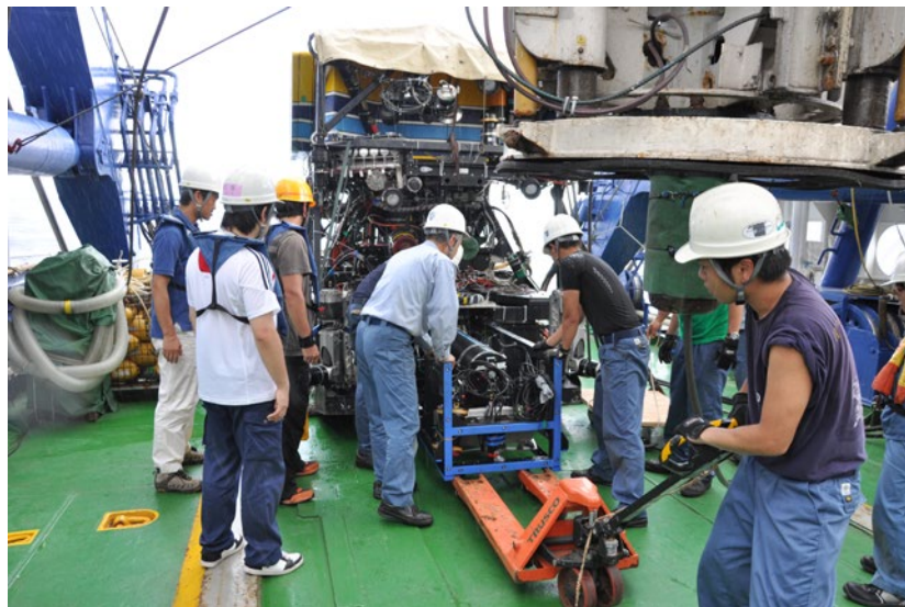
Fig: 5 Payload Skid being slid in to the payload bay of HyperDolphin
