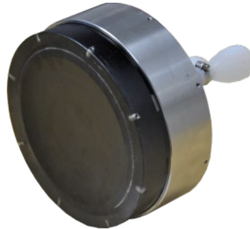
Fig: 6 Acoustic probe developed to measure manganese crust thickness.
